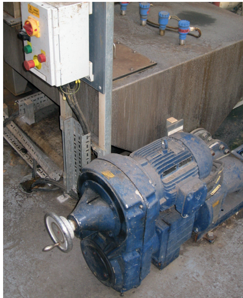
Previous control with level probes and mechanical speed variator
